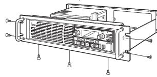
3 Disconnect the control cable from the channel module (original), then remove the front panel.
